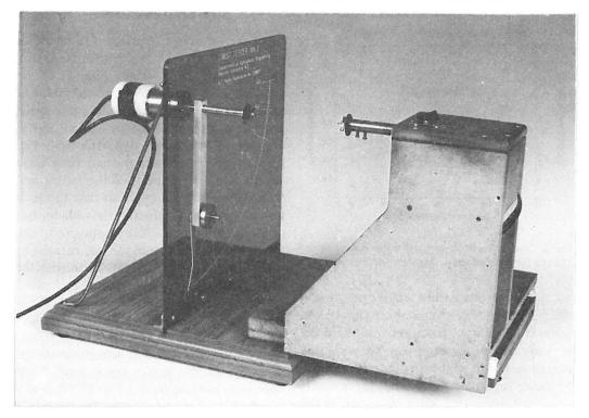
Fig. 4. Motor driven Twist Tester.
