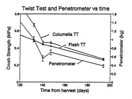
Fig. 2. Crush strength for kiwifruit tissue and columella, and penetrometer values, during storage (Orchard 2).
