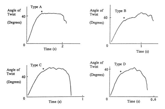
**Fig. 5.** Angle time curves for motorised twist tester. The bioyield point is indicated by \*. Type A - bioyield equal to maximum torque; Type B - torque falls then increases after bioyield; Type C - torque constant then increases after bioyield; Type D - no clear bioyield; value calculated from rotation (see text).
